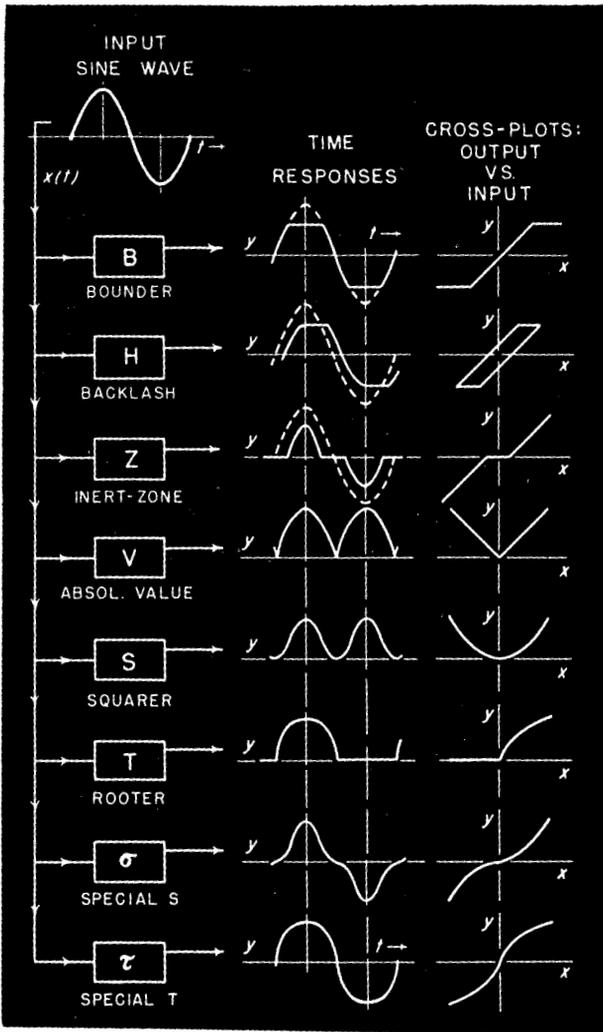
FIG. 3.—CHARACTERISTICS OF TYPICAL NON-LINEAR ANALOG COMPUTER COMPONENTS.
