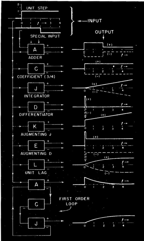
FIG. 2.—CHARACTERISTICS OF LINEAR ANALOG COMPUTER COMPONENTS.
