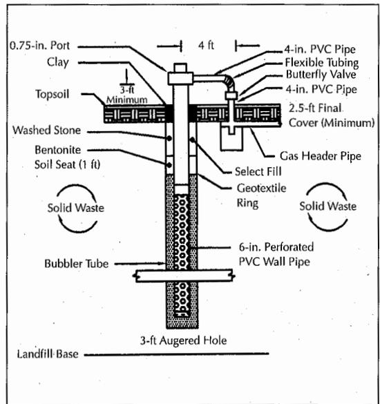
FIGURE 1. A typical LFG recovery well.
