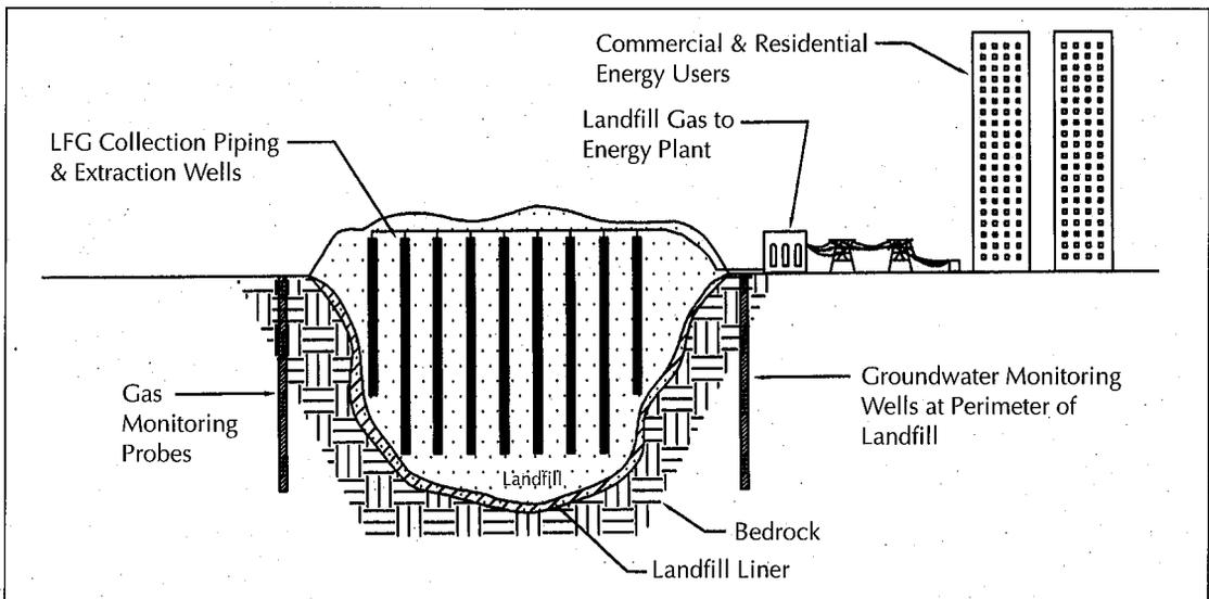
**FIGURE 2. A typical elevation of a LFG recovery system.**
