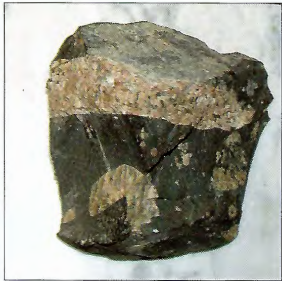
FIGURE 3-44. Gabbro dike from Porter Square Subway Station in Cambridge with fragment of granite. (Photo courtesy of Allen Hathaway.)
