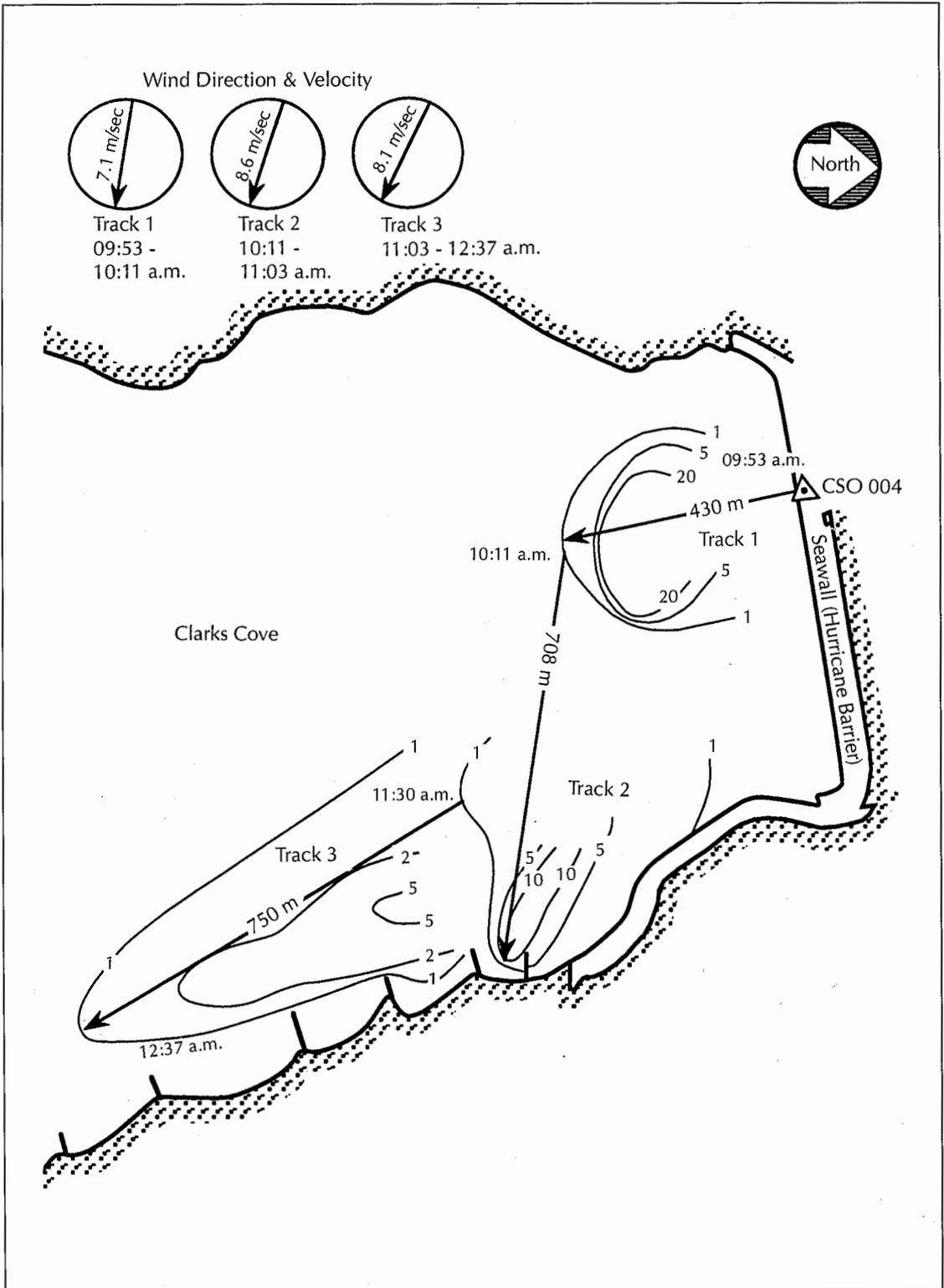
**FIGURE 2. Leading edge of dye plume from a CSO discharge on April 20, 1989, in Clarks Cove, New Bedford Harbor. Contours represent dye concentrations in parts per billion.**
