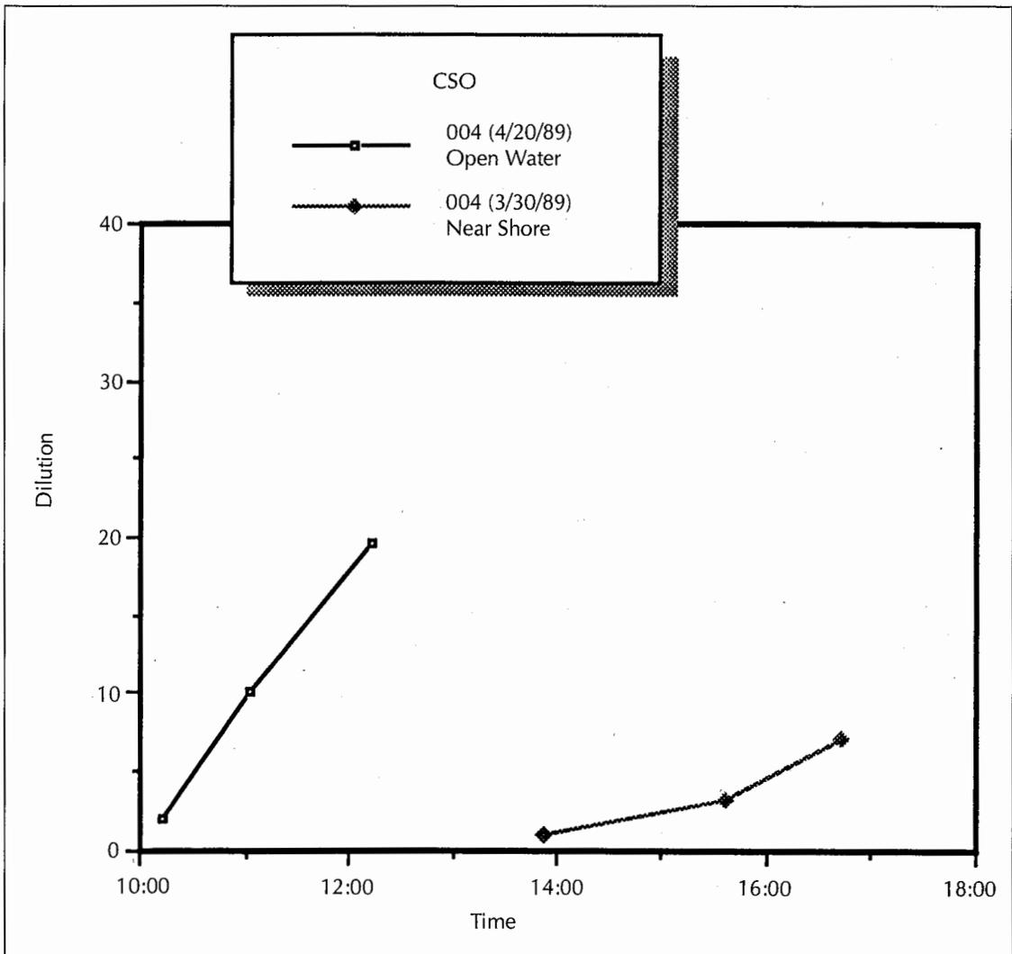
FIGURE 3. Dilution of CSO discharge in New Bedford Harbor as a function of time.
