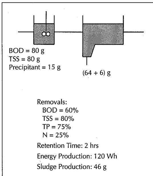
**FIGURE 5. CEPT sludge and energy production.**
