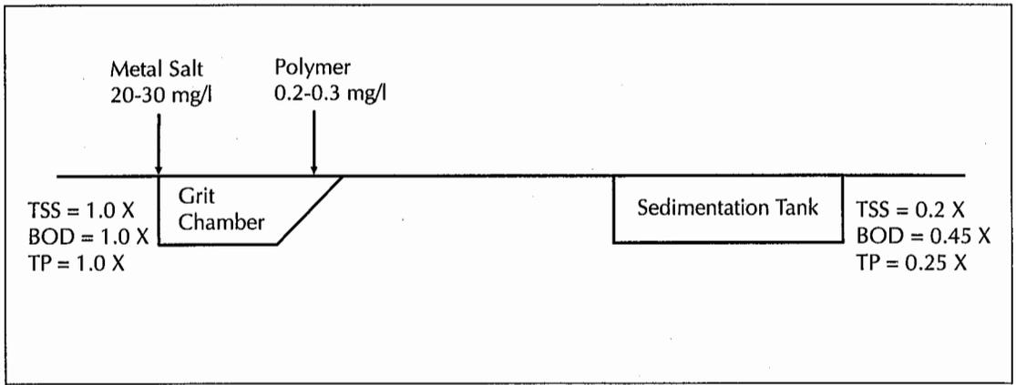
**FIGURE 1. Schematic of the CEPT process.**
