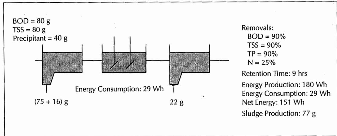
**FIGURE 9. Direct precipitation followed by an activated sludge process (sludge and energy production/consumption).**
