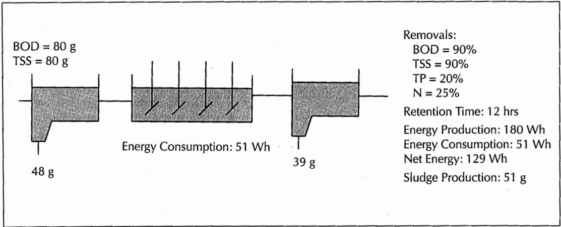
**FIGURE 7. Conventional primary treatment followed by an activated sludge process (sludge and energy production/consumption).**
