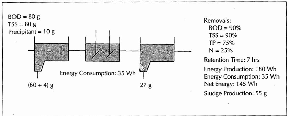
**FIGURE 8. CEPT followed by an activated sludge process (sludge and energy production/consumption).**
