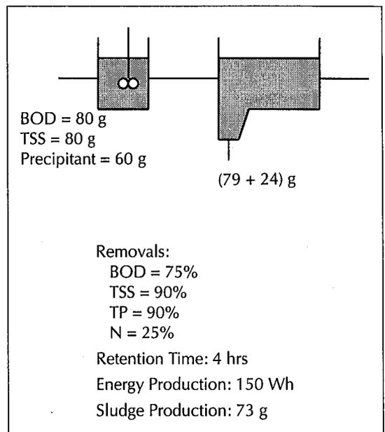
**FIGURE 6. Direct precipitation sludge and energy production.**
