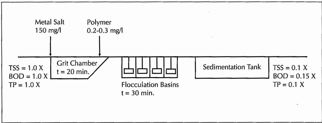
**FIGURE 2. Schematic of the direct precipitation wastewater treatment process.**
