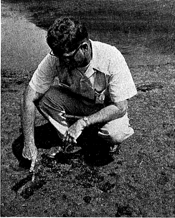
FIG. 33.—TEST HOLE SHOWING EXTENT OF OIL PENETRATION INTO RESERVOIR FLOOR.
