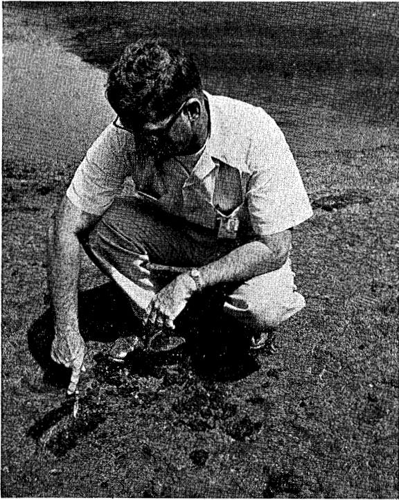
FIG. 33.—TEST HOLE SHOWING EXTENT OF OIL PENETRATION INTO RESERVOIR FLOOR.
