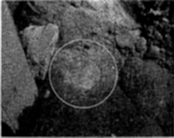
FIG. 7.—PHOTOGRAPH OF THE ROCK BELOW POINT NO. 1 IN FIG. 6. The circle indicates the depression caused by the pile point.
