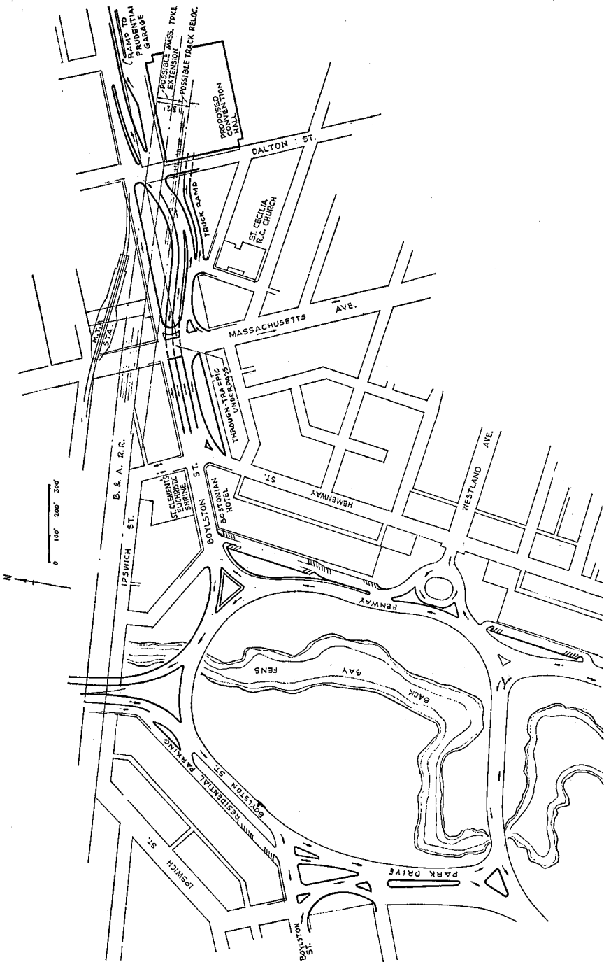
FIG. 12.—PROPOSED IMPROVEMENT FOR BOYLSTON STREET-MASSACHUSETTS AVENUE INTERSECTION, AND ON-STREET PARKING FOR RESIDENTIAL NEIGHBORHOODS AT THE FENS.
