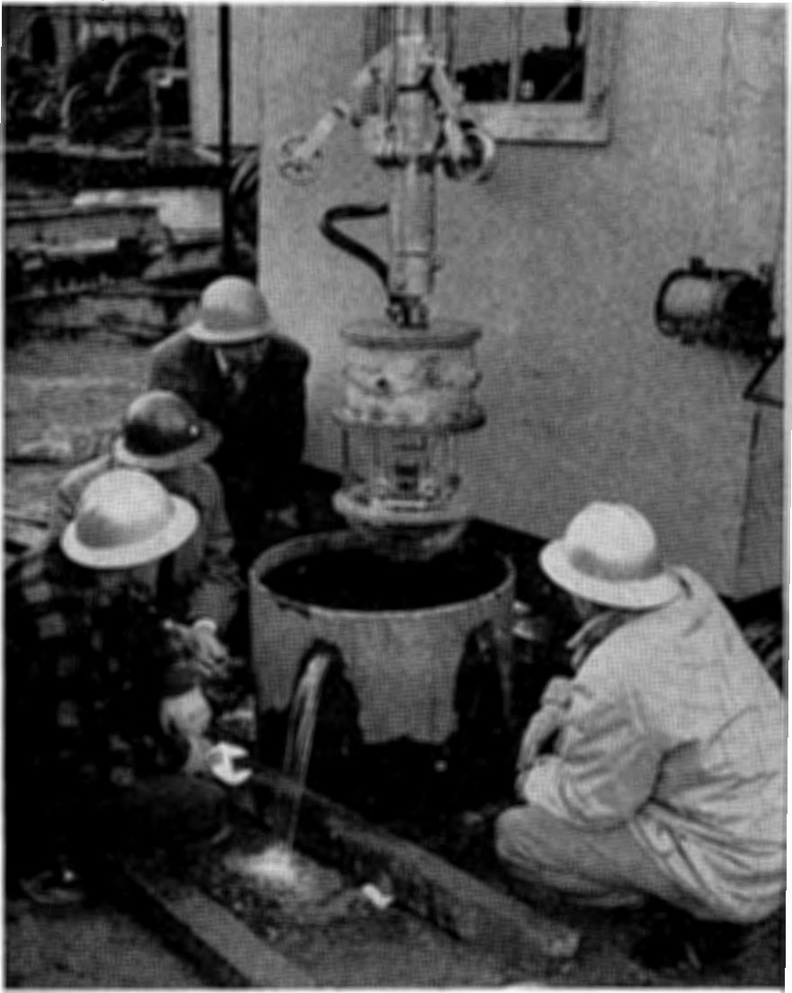
FIGURE 4.—UNDERWATER TELEVISION CAMERA DESIGNED TO OPERATE 160 FEET BELOW WATER SURFACE.
