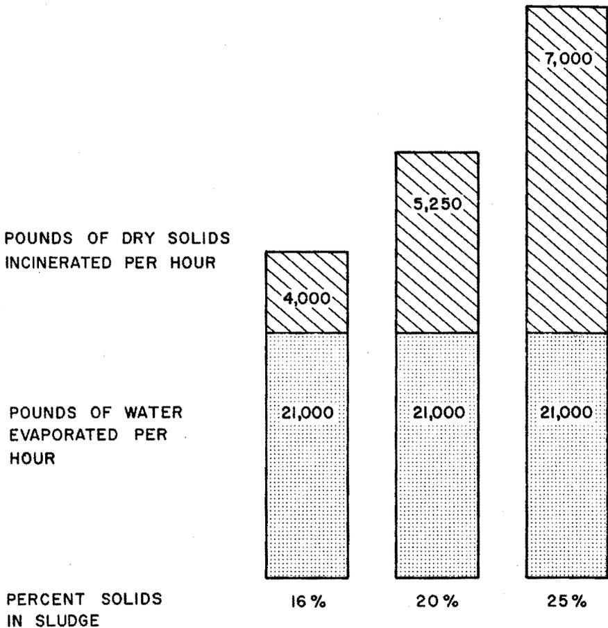
Fig. 6— Incinerator capacity.
