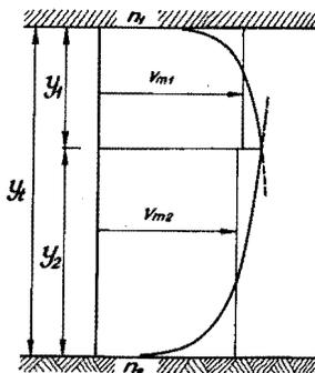
Fig. 10 — Theoretical velocity distribution. Definition sketch.
