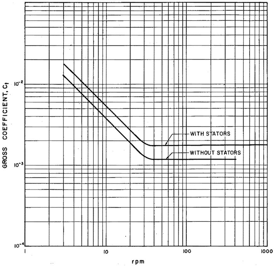
Fig. 4 — Gross drag coefficients for 4.4 in. sq. Rapid Mix Tank with water at 30°C.
