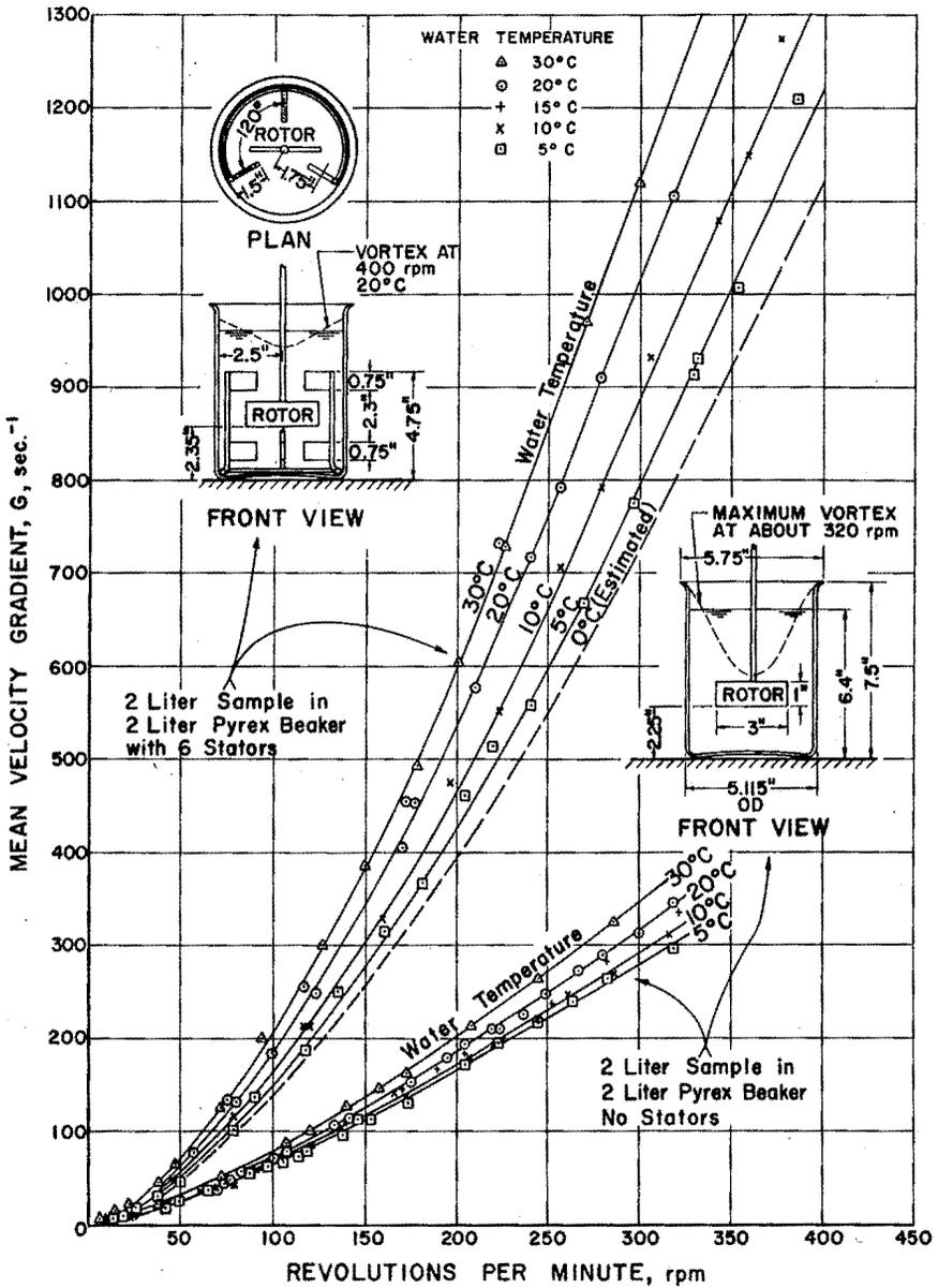
Fig. 1 — Velocity gradient calibration curves for water.
