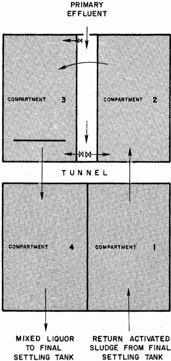
Fig. 7 — Plan of one aeration tank.
