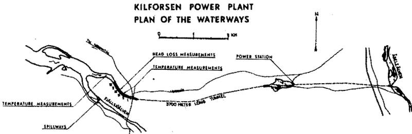
Fig. 13 — Plan of the Kilforsen Hydro Power Plant.
