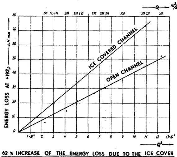
Fig. 20 — Head losses with and without an ice cover related to a common stage.
