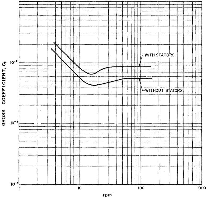
Fig. 7—Gross drag coefficients for 1 ft. sq. tank 1 ft. deep with water at 30°C.
