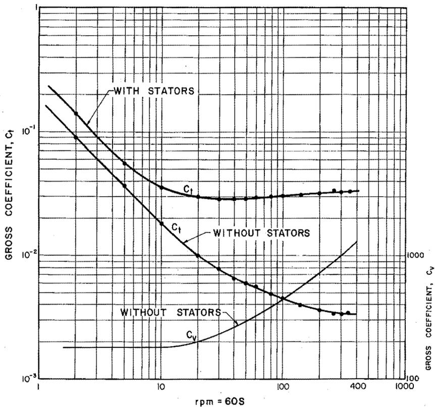
Fig. 3 — Gross drag coefficients for 2-Liter Beaker with water at 30°C.
