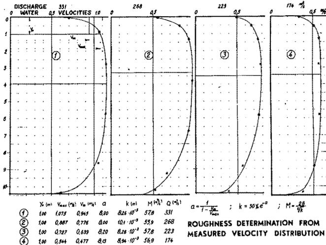
Fig. 17 — Vertical velocity distribution with 4 different flow rates.
