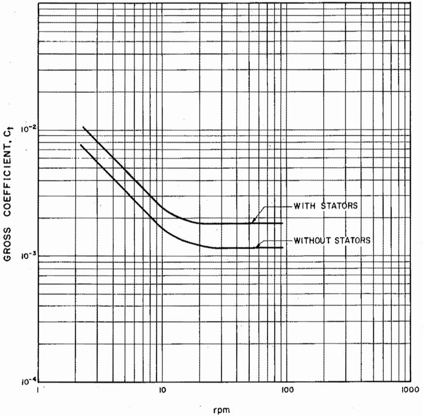
Fig. 6—Gross drag coefficients for second 8 third 1 ft. sq. tank, 3 ft. deep, water at 30°C.
