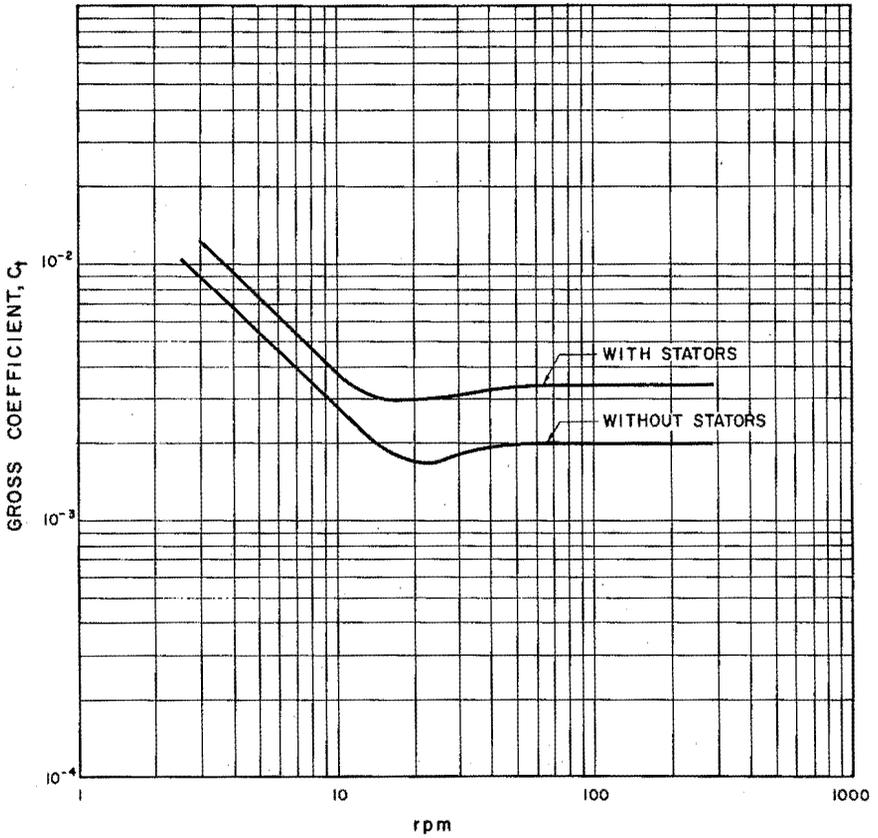
Fig. 5—Gross drag coefficients for first 1 ft. sq. tank 3 ft. deep with water at 30°C.
