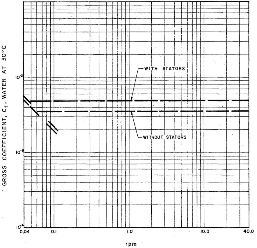
Fig. 8— Estimated position of tangents to curves for gross drag coefficients for Billerica, (Mass.) rapid mix.
