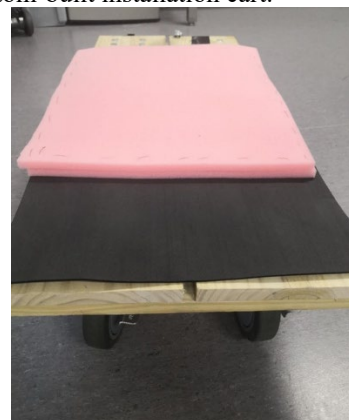
Figure 12. Two-layer cushion on installation cart.
