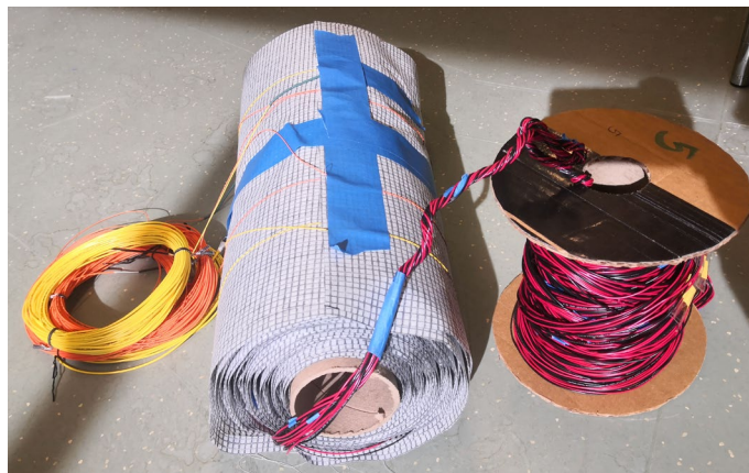
Figure 9. Manufactured sensing textile in a roll.
